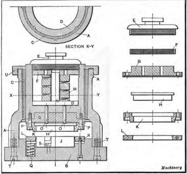
Fig. 2. Sub-press Die of Typical Design
